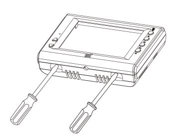
Insert the awl into the slot and pry up the front part of the panel to open it.
