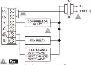
1.Please set on the heat pump system first. 2.Please set the valve as heating/cooling system
