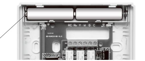
Insert 2 AA Alkaline batteries (not included). High quality alkaline batteries are recommended.
