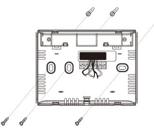
For horizontal mount put one screw left and one screw right.
